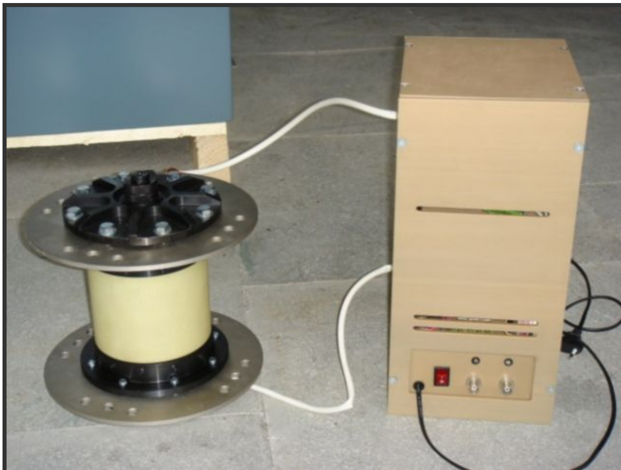
Fig. 12. RSD commutator 300 kA, 25 kV DC with control generator
